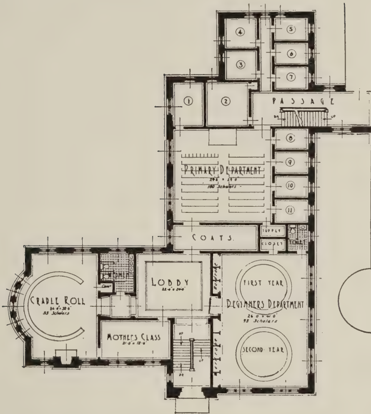
MAIN FLOOR PLAN OF NEW EDUCATIONAL BUILDING OF ELM PARK M. E. CHURCH, SCRANTON, PA., SHOWING CLASSROOMS FOR PRIMARY DEPARTMENT
